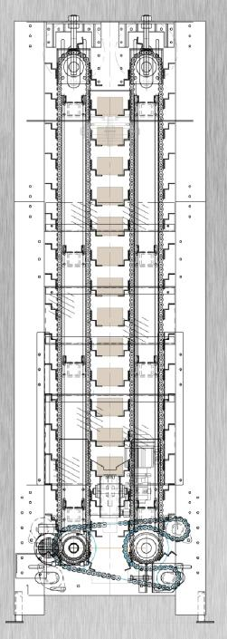
Primarily used for accumulating heavy or large items (cases). Our angle accumulator can solve unique accumulation issues where budgetary constraints are an issue. Dillin's Angle Accumulator is an economical alternative to Over-the-Top® technology while maintaining many of the features and benefits.
